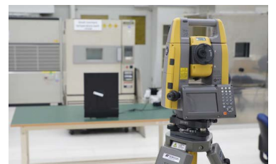
Auto-tracking durability test against rotating object.
