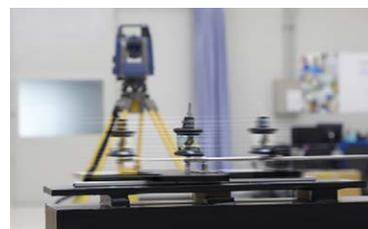
Auto-tracking test under high speed vibration conditions
