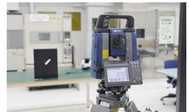
Auto-tracking durability test against rotating object.
